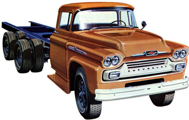
1958 Spartan 80 or 100 Series Tandem Again the Hood emblem notes a V-8 engine; either a 175 HP HD Super Taskmaster V-8 (80 Series), or 230 HP Workmaster V-8.
