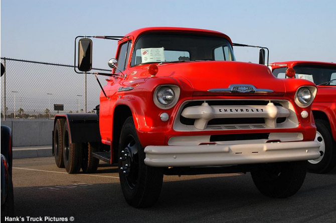
1955-57 Spartan 1000 Tandem Hood emblem notes a V-8 engine; either a 155 HP Taskmaster V-8, or 162 HP Turbo-Fire V-8.
